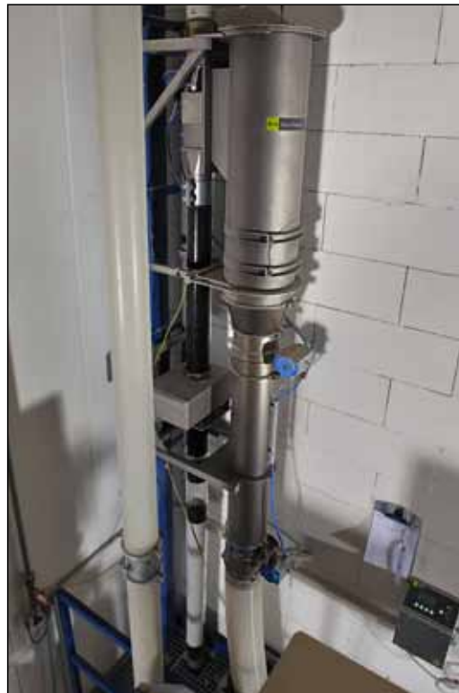
GF 4000 metal separation systems installed in vertical pressure pipes.
